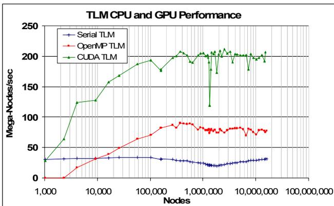
Fig. 5 Performance comparison between the traditional CPU and GPU TLM algorithms.
