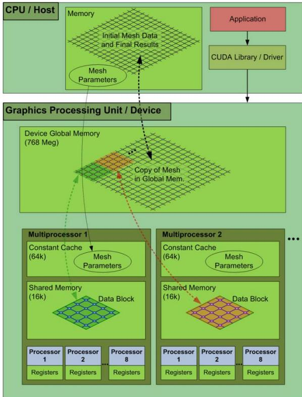
Fig. 1 The host-device relationship between a computer's CPU and GPU. Also depicted is the memory model of the NVIDIA GeForce 8800 GTX Ultra GPU used in this project.
