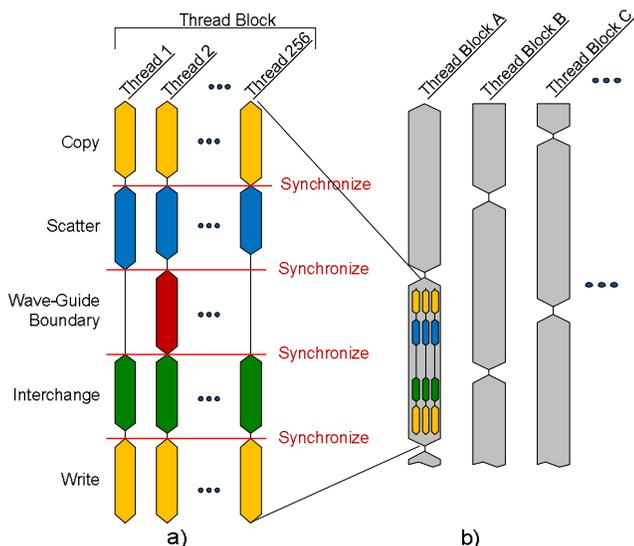
Fig. 2 a) Synchronization of computation stages within a thread block can be handled directly by a GPU sync function. b) Synchronization among thread blocks must be handled by other means.
