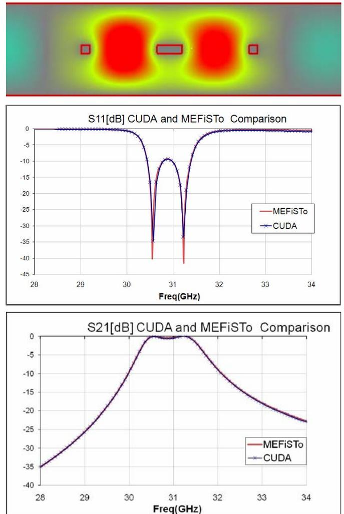
Fig. 6 The field distribution, return loss and insertion loss of a bandpass filter in a WR28 waveguide. The dimensions of the inductive obstacles are  $0.6465\text{mm} \times 0.6465\text{mm}$  and  $0.6465\text{mm} \times 1.9340\text{mm}$ . The spacing between the obstacles are  $5.172\text{mm}$ .
