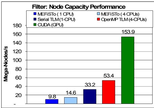
Fig. 7 Performance of various TLM implementations for a bandpass filter in a WR28 waveguide.
