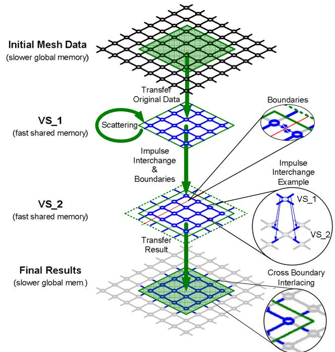
Fig. 3 Parallel computational iteration by thread block.
